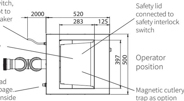
2 m cable for connection to main electrical safety switch, see (1) next page, but not to earth leakage circuit breaker
